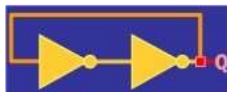
Fig.1: Simplest realization of feedback circuit
